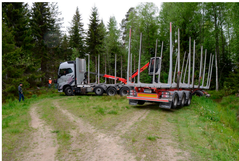
Figure 7. HCTs (76 t with crane) need larger turning places on forest roads (photo: Markus Strandström).
